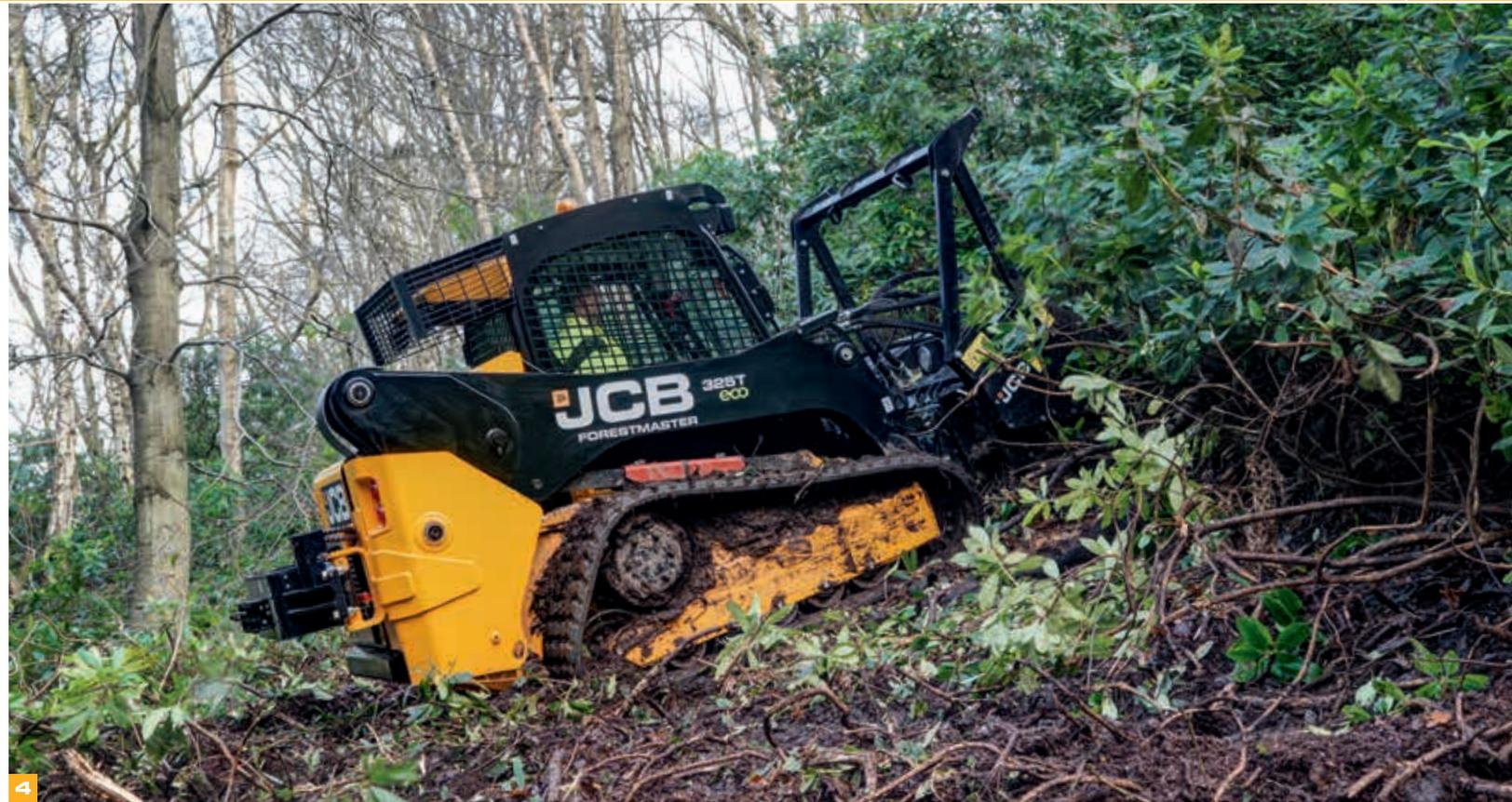
4 Level 2 Falling Object Protection Structure (FOPS) shields the operator from danger above while left and right hand steel mesh provides peripheral protection.
