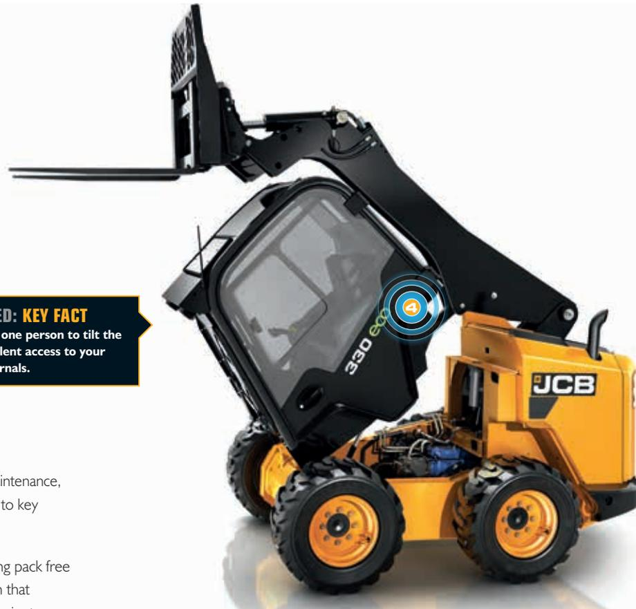
**4** When it comes to more complex maintenance, our tilting cab design ensures easy access to key components.
